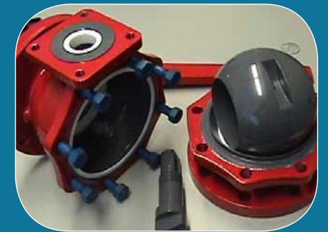
DND valves blasting and coating with xylan
