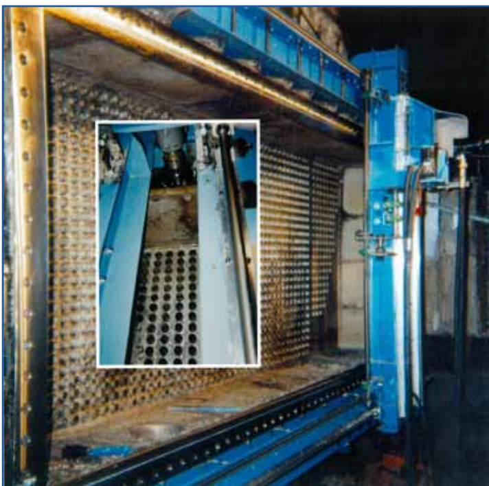
Large Diameter Machining OD Portable Boring Bar Inside Diameter Machining.
