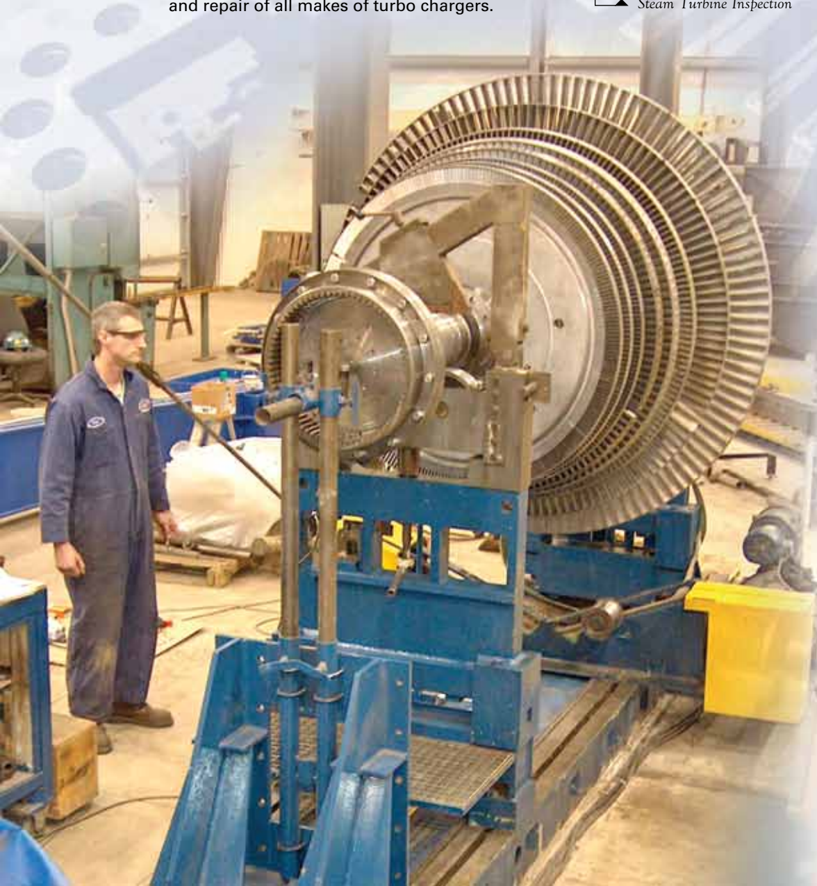
▲ Steam Turbine Inspection
